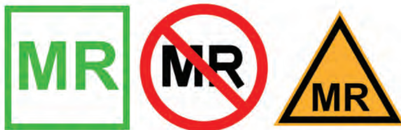
■ FIGURE 13-46 MR labeling includes on the left, MR safe materials that have been found not to interact with the strong MR field or disrupt operation; in the middle, NOT MR safe labels that contraindicate bringing materials with this designation past Zone 2 (see discussion later in this section; on the right, more consideration required before bringing such labeled objects into the scan room).
